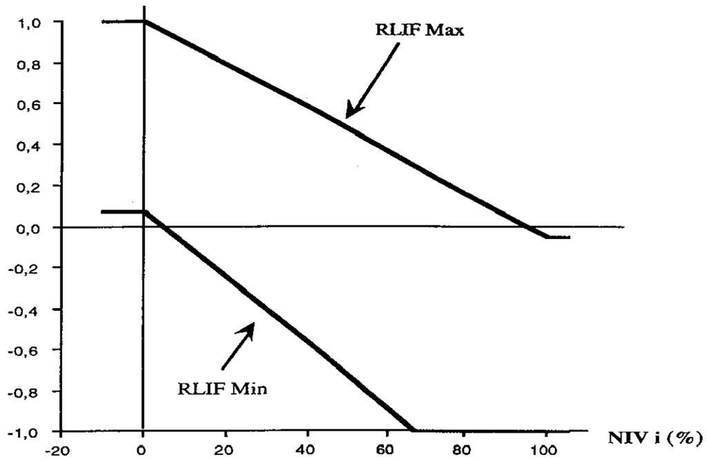
Figure 5.2: Inferior and Superior Limits on LZC Valve Opening Demand
